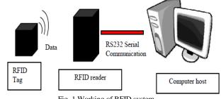
Fig. 1 Working of RFID system
