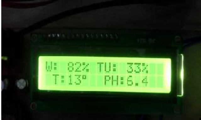
Figure 7. Sensors Readings on LCD (for water sample1 in observation table )
