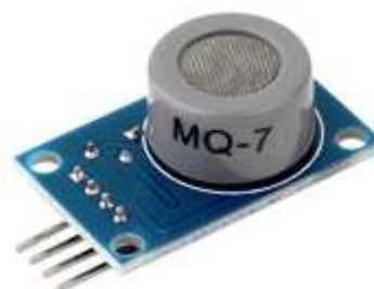
Fig. 2. Carbon monoxide sensor
