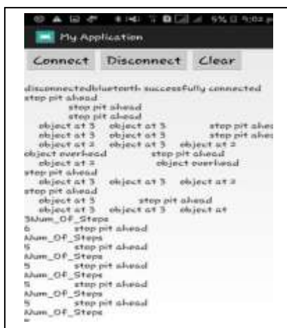
Fig. 8. Snapshot showing data stream received through Bluetooth as voice output.
