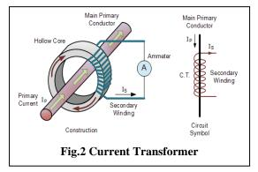
turn coil of the heavy duty wire wrapped around the core or just as conductor or the bus bar placed through the central hole as shown in the Fig.2.Due to such type of arrangement, the current transformer is often referred to as the series transformer as the primary winding, which never has more than a very few turns, is in series with the curent carrying conductor supplying the load
