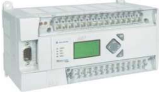
Figure 6: programmable logic controller (PLC)
