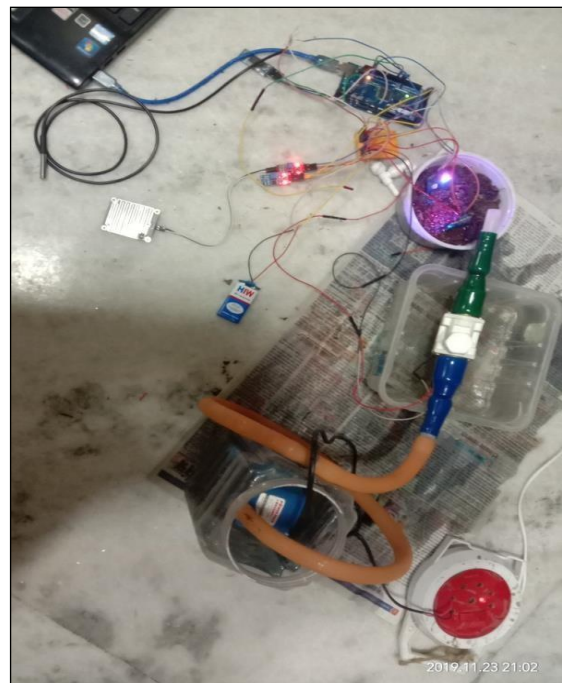
4. Value from soil moisture sensor is less than 700 so solenoid valve will remain off.
