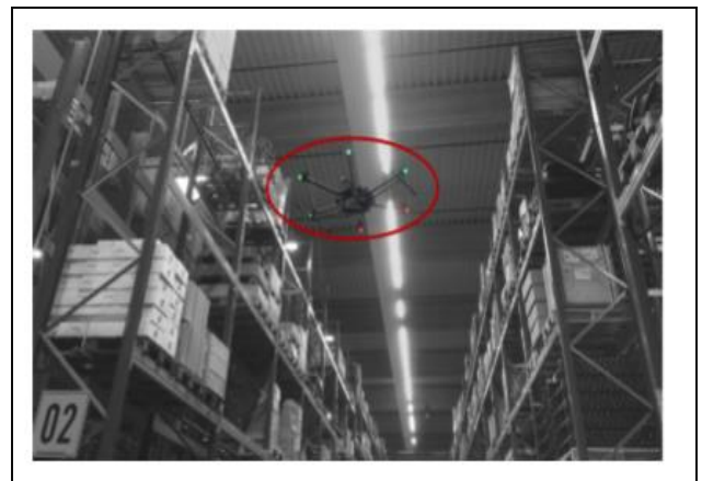
Fig.3 MAV performing the inspection task in warehouse
