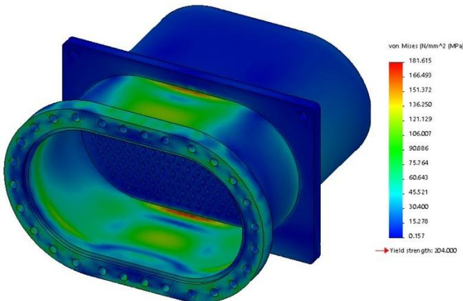
Fig. 5 von Mises stress plot of obround flange (view-1)
