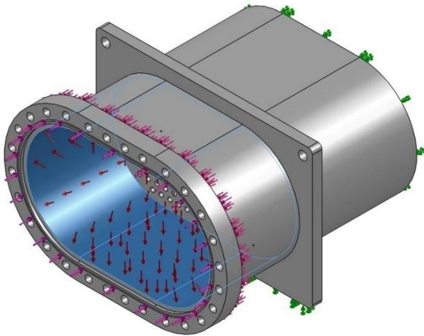
Fig. 4 Boundary conditions and loading
