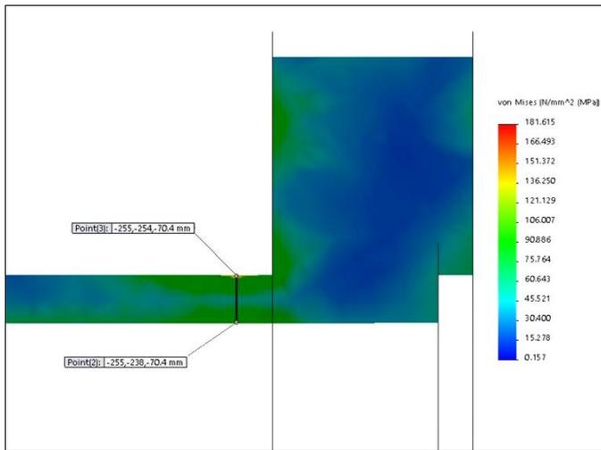
Figure 11. Stress classification line near flange to shell transition
