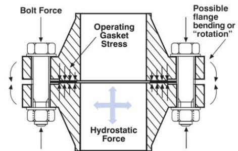
Fig. 1 forces acting in a bolted flange joint assembly
