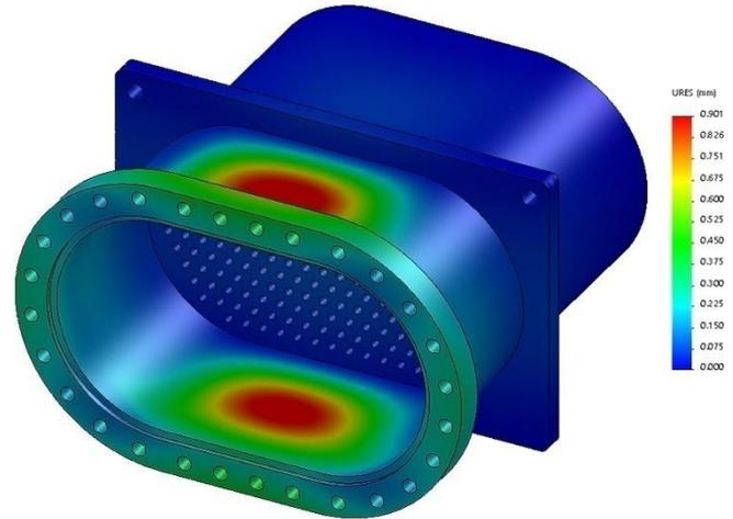
Fig. 7 Deformation plot of obround flange
