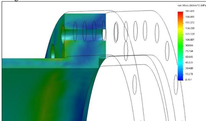
Fig. 8 Stress concentration zone in flange
