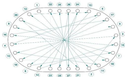
Figure 13. Bolt tightening sequence
