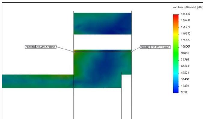
Fig. 9 Stress classification line through flange
