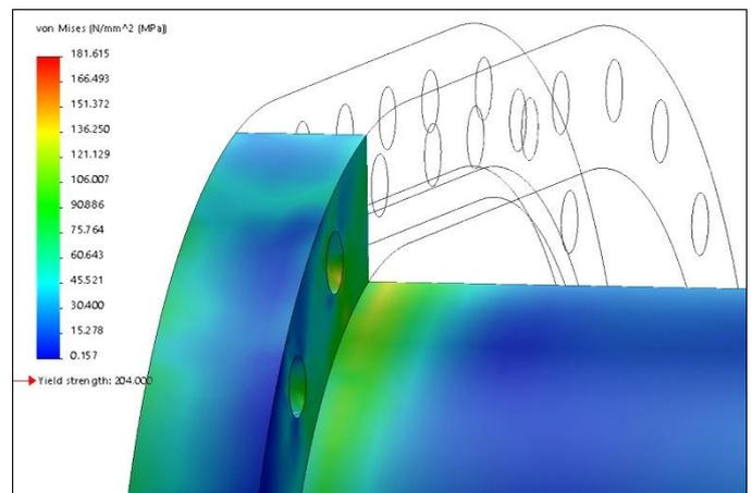
Figure 10. Stress concentration zone near flange to shell transition
