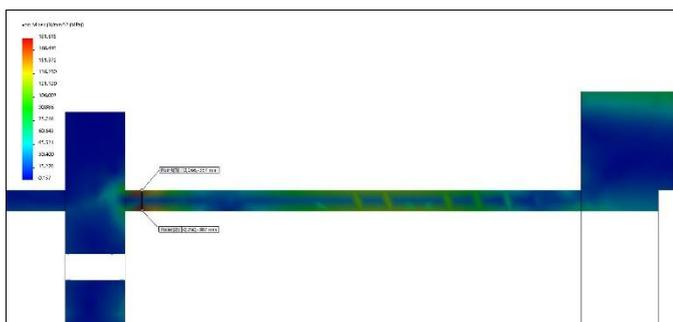
Figure 12. Stress classification line on shell
