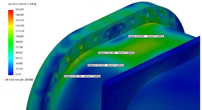
Fig. 6 von Mises stress plot of obround flange (view-1)
