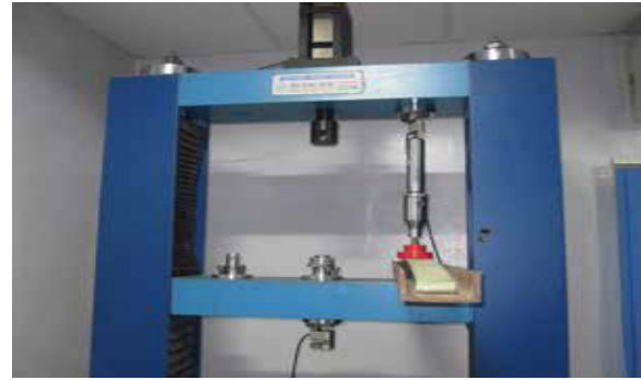
Fig.1 Experimentation set up of composite leaf spring
