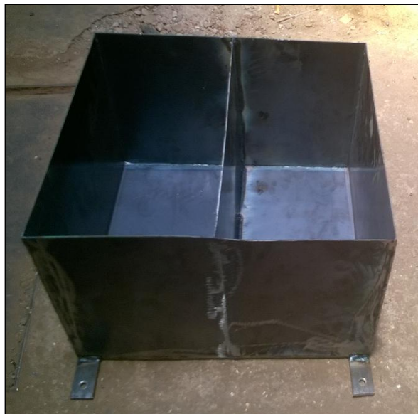
Fig. 2 Oil tank divided in two chambers
